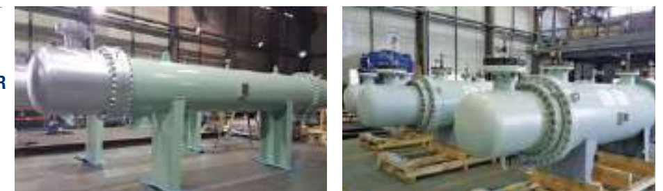
RECYCLE GAS COOLER AND AFTER COOLER
