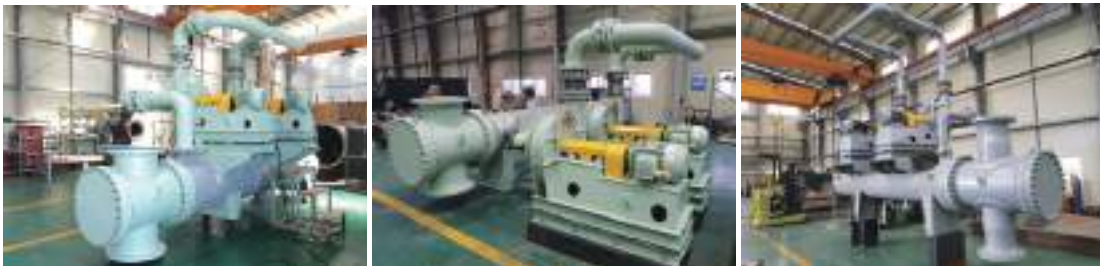
FAN BLOWER EXHAUST TYPE GLAND STEAM CONDENSER
