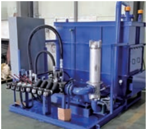
Oil Flushing Equipment
