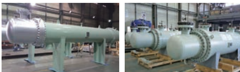
RECYCLE GAS COOLER AND AFTER COOLER
