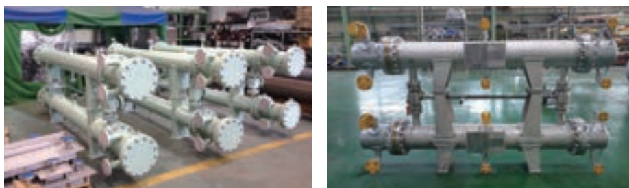
LUBE OIL COOLER
